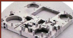
Figure 5.13 The first was precision computer-controlled milling. This base casting is from a Sony BVH-2000 Type C one-inch VTR. Long wraps meant
