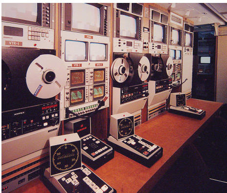
Figure 5.18 Two mainstay one-inch VTRs that were used throughout the '80s and into the '90s: Sony's BVH-2000 onboard a CBS truck (left), and Ampex VPR-2s on the right, with their "slo-mo" controllers sitting on the desk in an ABC truck. TBCs for these machines were generally separate boxes, such as can be seen below each BVH-2000 and slightly protruding from the racks. The tops of the TBCs for the VPR-2s are peaking out behind the countertop and directly below the VTR. (Source: A.F. Associates)
