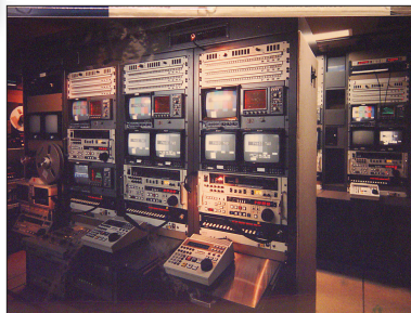
Figure 5.18 Two mainstay one-inch VTRs that were used throughout the '80s and into the '90s: Sony's BVH-2000 onboard a CBS truck (left), and Ampex VPR-2s on the right, with their "slo-mo" controllers sitting on the desk in an ABC truck. TBCs for these machines were generally separate boxes, such as can be seen below each BVH-2000 and slightly protruding from the racks. The tops of the TBCs for the VPR-2s are peaking out behind the countertop and directly below the VTR. (Source: A.F. Associates)
