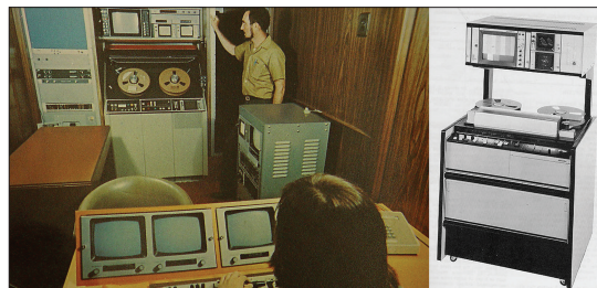
Figure 5.15 At left is RCA's last model quad on a truck in the early 1970s, the TR-600. Ampex brought one more version out in the mid-70s. This VTR found its way onto a number of trucks, large and small. Its architecture was such that the tape transport could be separated from the rest of the electronics. This meant that this quad could actually be put on a table. Far right: the AVR-2.
