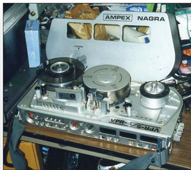
Figure 5.19 Sony and Ampex, along with Nagra, offered portable one-inch VTRs. From the mid-70s on there were 3/4-inch Umatic portables, but the quality was far from what the one-inch format could provide. (Source: Tim Stoffel)
